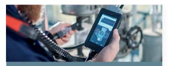
Digital ultrasonic testing device SONAPHONE®
